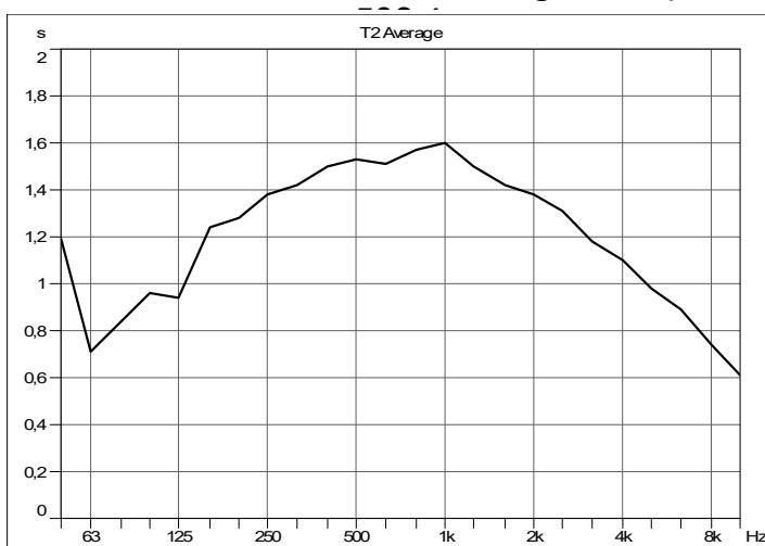
Fig.5. Reverberations time values in the secondary sound field for sample No 506-6.
